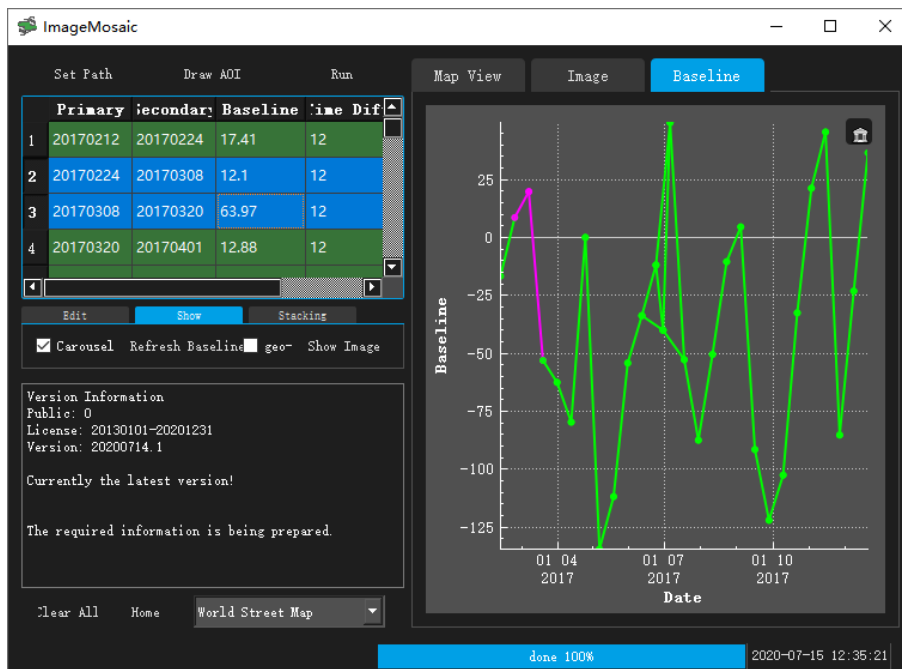
Fig. 7 Interferometric Configuration and Mosaic Tool User Interface – Baseline
